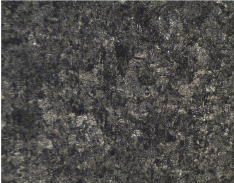
**Fig. III.11** 100Cr6 recuit X20
