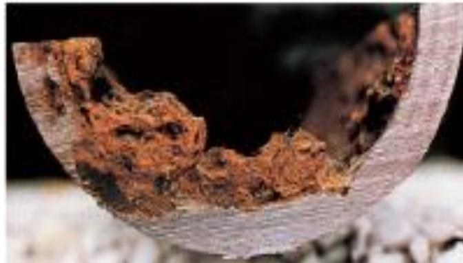
*Figure I.4: Corrosion uniforme [2]*
