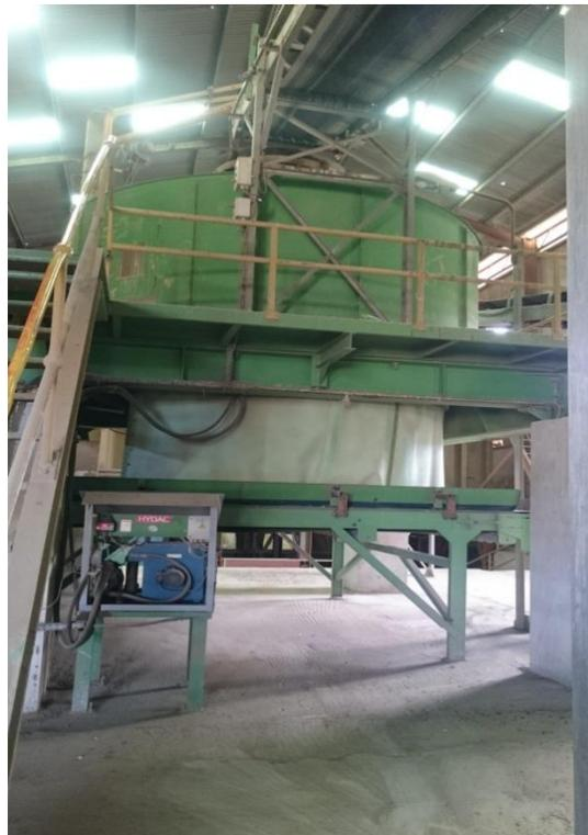
Figure I-9: Broyeur A Meules
